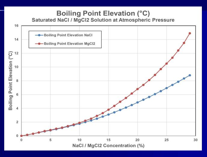
Salt solution boils at a temperature that is higher than the temperature of water at the same pressure.
