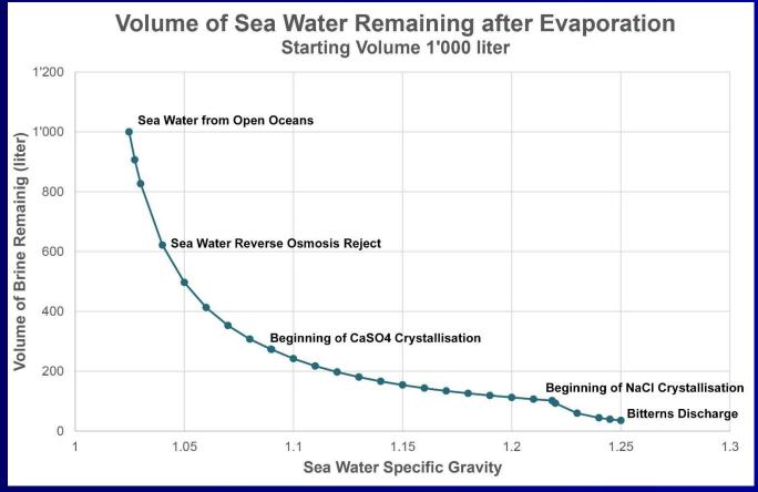
When sea water evaporates or water is being removed in a desalination process, the volume is reduced and the concentration is rising. 96.45% of water is removed to crystallise 23.05 kg of NaCl from the original 1'000 I of sea water
