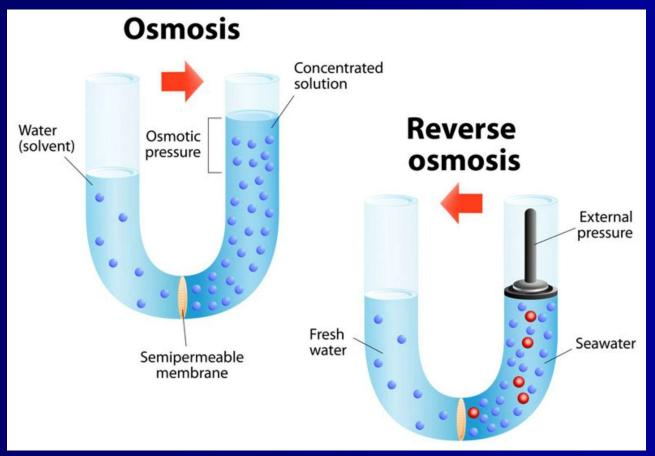
Concentrated salt solution pulls water through membrane from diluted solution up to the point of equilibrium pressure called the osmotic pressure.
